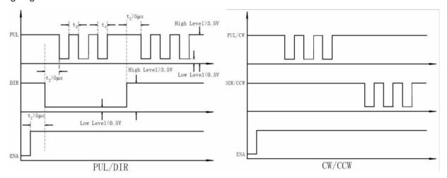
Figure 11: Sequence chart of control signals
