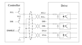
Figure 3: Connections to open-collector signal (common-anode)
