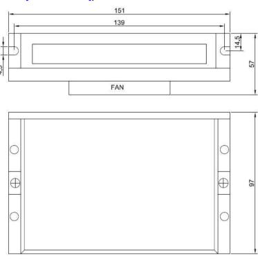
Figure 1: Mechanical specifications
