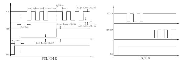
Figure 6 Sequence chart of control signals
