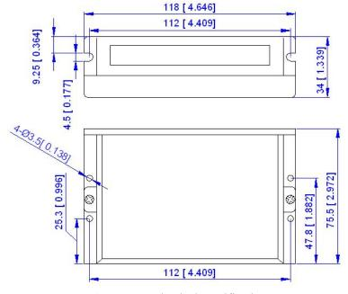
Figure 1 Mechanical specifications
