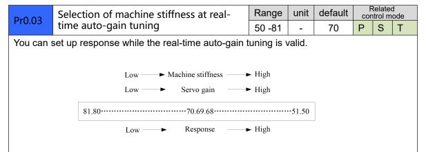
**Notice:** Lower the setup value, higher the velocity response and servo stiffness will be obtained. However, when decreasing the value, check the resulting operation to avoid oscillation or vibration.
