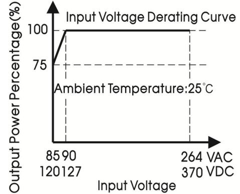
Note: 1. With an AC input voltage between 85 - 90VAC and a DC input between 120 - 127VDC the output power must be derated as per the temperature derating curves;
