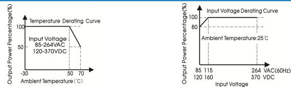
Note: 1. With an AC input voltage between 85-115VAC and a DC input between 120-160VDC the output power must be derated as per the temperature derating curves;
