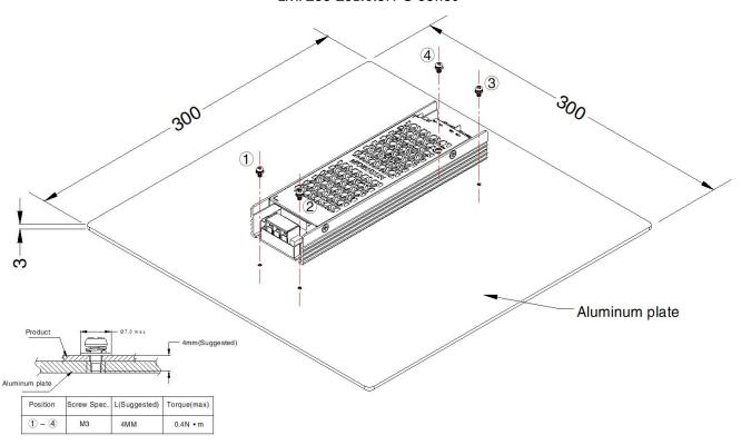
Note: 1. In order to meet the "Derating Curve", the product testing must be installed onto an aluminum plate. The size of the suggested aluminum plate is shown as above. And for optimizing thermal performance, it is necessary to apply thermal grease on the bottom of the product.
