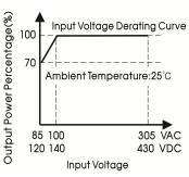
Note: 1. With an AC input voltage between 85-100VAC and a DC input between 120-140VDC the output power must be derated as per the temperature derating curves;
