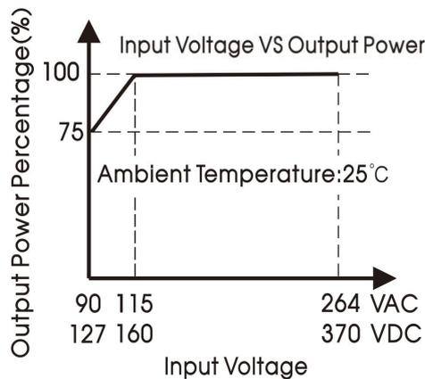
Note: With an AC input voltage between 90 - 115VAC and a DC input between 127 - 160VDC the output power must be derated as per the temperature derating curves
